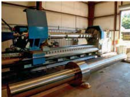
Stepped shafts or unusual shapes are easily machined with a 5-axis CNC lathe with live tooling.
