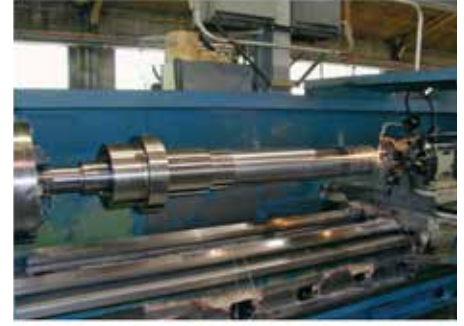
Sub-assembly with interference fit prior to or after machining is available.
