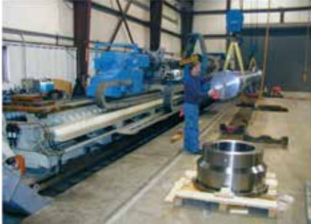
Large bar CNC threading to B/P tolerances or matched to mating nut.
