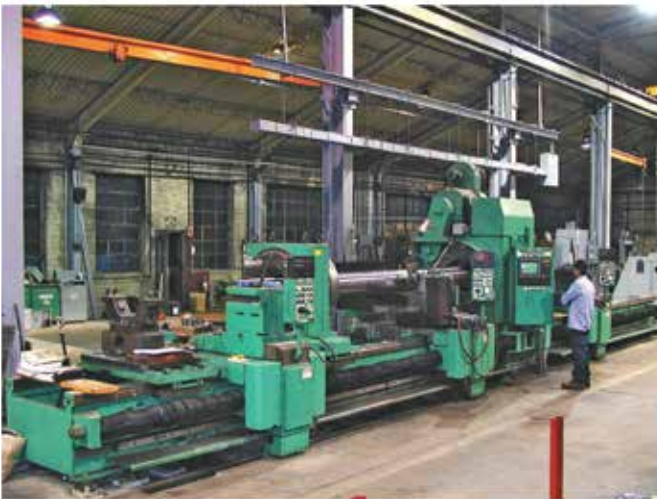
Close tolerance CNC turning measured with temperature compensating laser.
