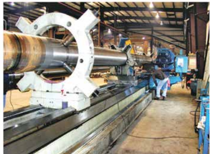
Long shaft CNC machining with live tooling for same setup secondary operations.
