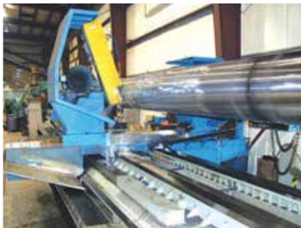
Same machine polishing helps achieve close tolerance and finishes in one step.
