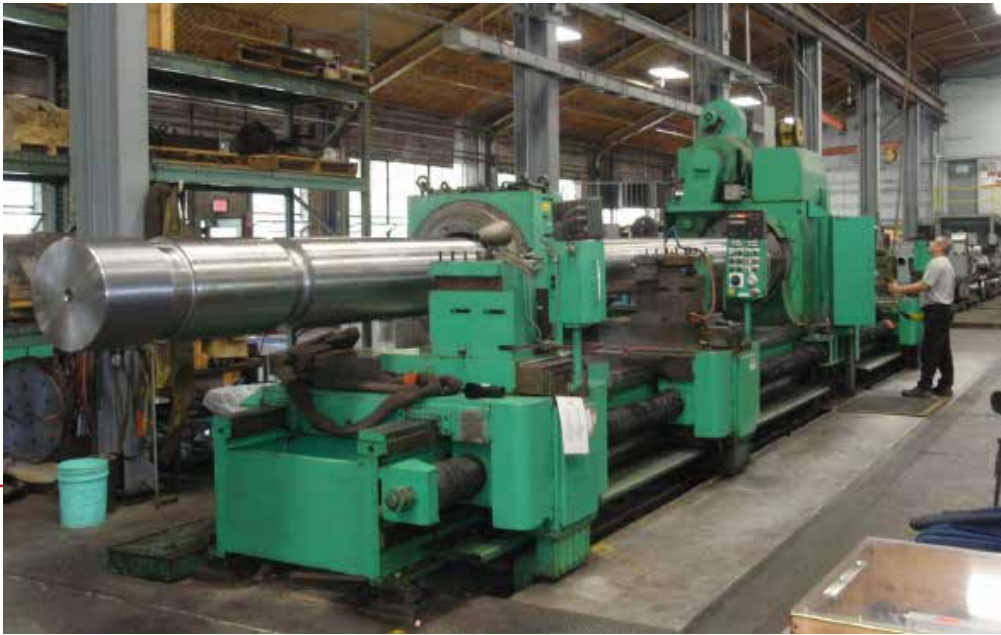
Shortening machined area for rigidity with Center Headstock CNC Lathe
