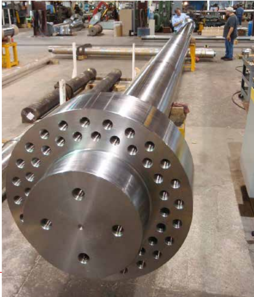
8000T forge press column, 40,000 lbs
