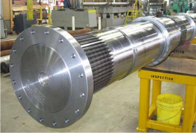
Press Shaft with Induction hardened ppines
