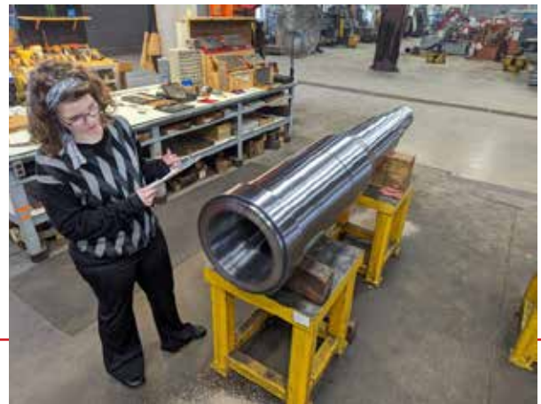
Axial roll sleeve with laser hardened ID tapers
