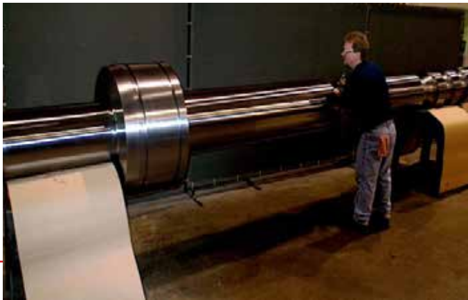
Final inspection of precision configuration profile
