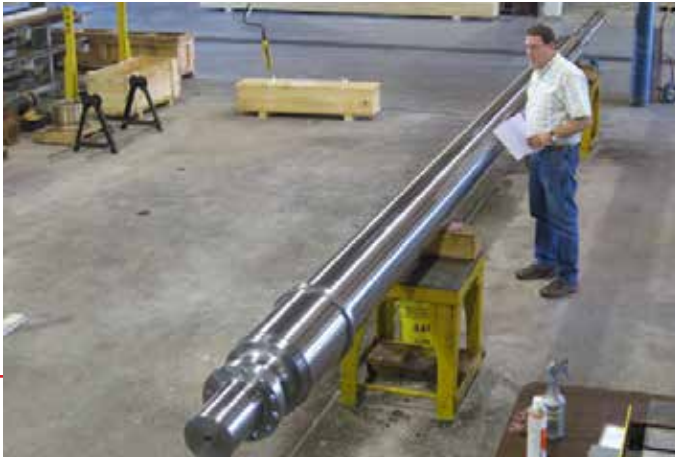
6-pc fabricated mixing screw shaft for carbon paste processing
